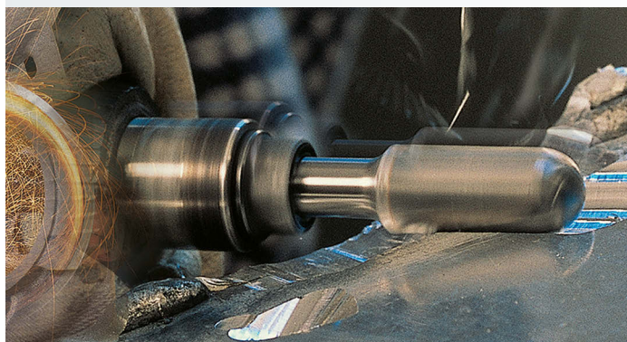
Example using burr with Z9 cut
